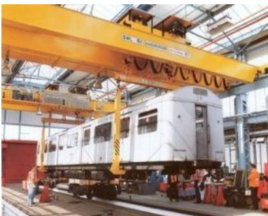
Overhead Gantry Crane
